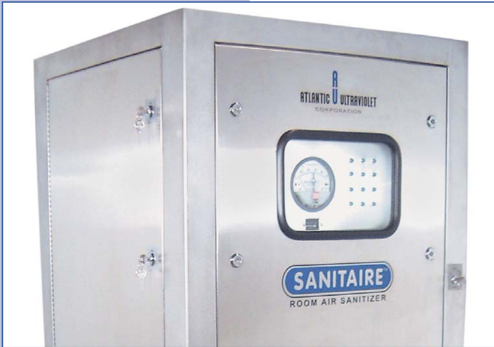
Figure 3 - Sanitaire® RSM2680 (shown) The Model RSM2680 Room Air Sanitizer is mobile, and requires no professional installation. Simply roll the fixture into the occupied area to be treated, and plug into an appropriate power source. When in operation, air is drawn into the fixture through the four louvered Filter Panels, located around the base of the fixture. The air passes into the exposure chamber, where it is irradiated by twelve (12) germicidal ultraviolet lamps. The air then passes out of the fixture, through the louvered Exhaust Panel, located on the top of the fixture.
